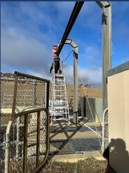
Image: Engineer carrying out flexion testing on the Linnburn Gates Gantry as part of the certification.
